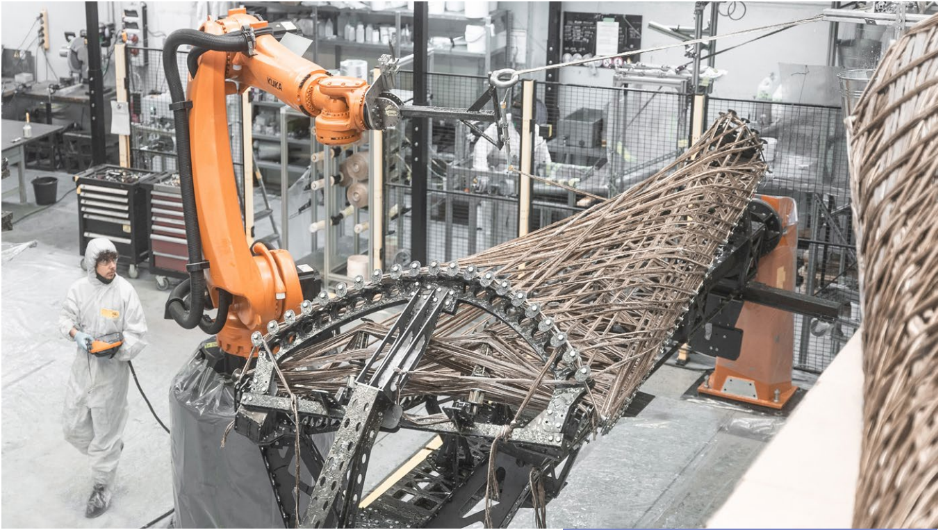
The robotic manufacturing process at FibR GmbH. Photo: IntCDC, University of Stuttgart / Robert Faulkner
